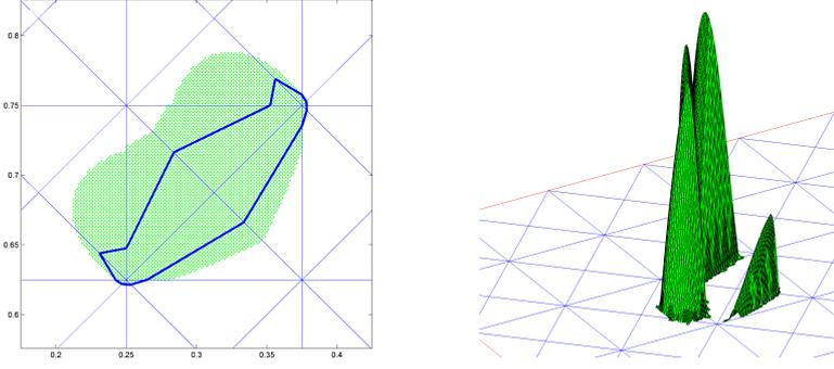
FIGURE 2.  $u_a$  active set: blue by  $u_h^\gamma$ , green by  $\tilde{u}^\gamma$  (left), integrand  $(\tilde{\lambda}^\gamma + \lambda_h^\gamma)(u_h^\gamma - \tilde{u}^\gamma)$  with support on symmetric difference of active sets (right).
