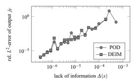
Fig. 2 Relative error between reduced and unreduced problem at the fixed frequency  $5 \cdot 10^9$  [Hz].
