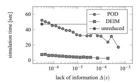
Fig. 3 Time consumption for simulation runs of Fig. 2. The horizontal line indicates the time consumption for the simulation of the original full system.
