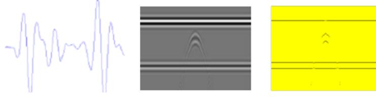
Figure 2. Left to right: a-scan, b-scan, deconvolved b-scan (preprocessed data)
