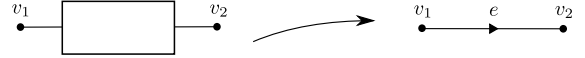
Figure 7: Deriving the underlying graph of a capacitance, conductance, ideal diode, PN-junction diode, inductance, resistance, or sources.
